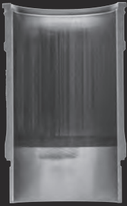
Severely Scuffed Liner
