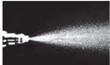
Injector spray pattern after P.i. treatment.
